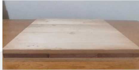
Fig. 1. Three layer CLT, central layer impregnated with PCM [3].
